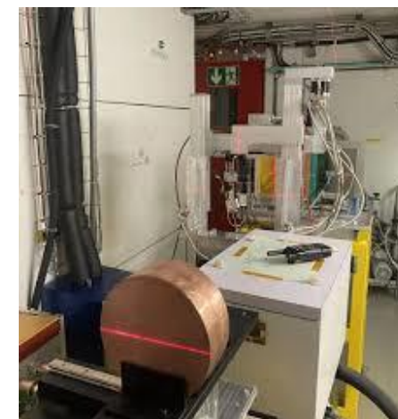
Sensor mounted for irradiation at CERN'S IRRAD facility
