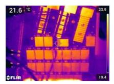
Before the modules were switched , temperatures ranged from 19.4 - 23.9  $^{\circ}\text{C}$
