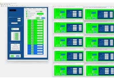
☐ Integration of HV to DCS fully operational enabling remote use, can operate all 54 modules, change over current protection, voltages,
