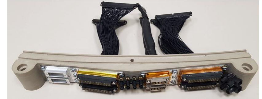
All sections of outer ring will be pre-assembled with services. First prototype shown in picture.
