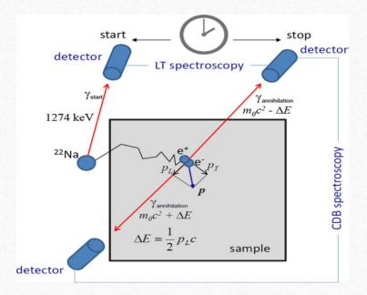
Sample-source sandwich arrangement for the registration of the birth and annihilation photon as start and stop signals is shown in figure 6 [4].
