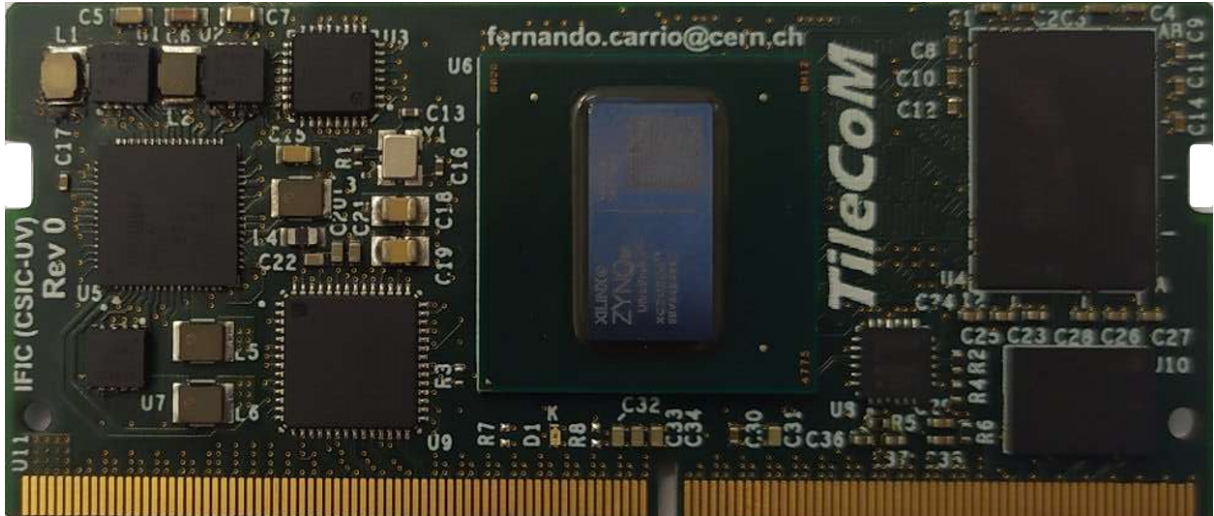
Figure 3: The Tile Computer On-Module (TileCoM)
