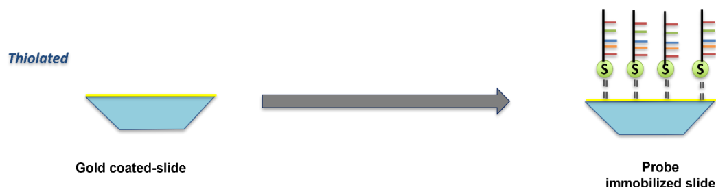
Figure 2: A simplified diagram of the immobilized thiolated DNA probes on the sensor chip surface.
