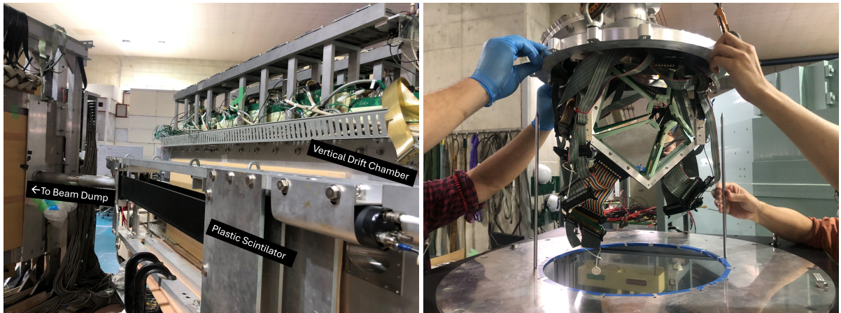
Figure 1: ( Left ): The focal plane detection system, with plastic scintillators positioned behind the vertical drift chambers. The zero-degree beam line is visible, passing within centimeters of the detectors. ( Right ): The cherry blossom-shaped SAKRA DSSSD array prior to installation in the scattering chamber. It covers approximately 25% of the downstream solid angle.
