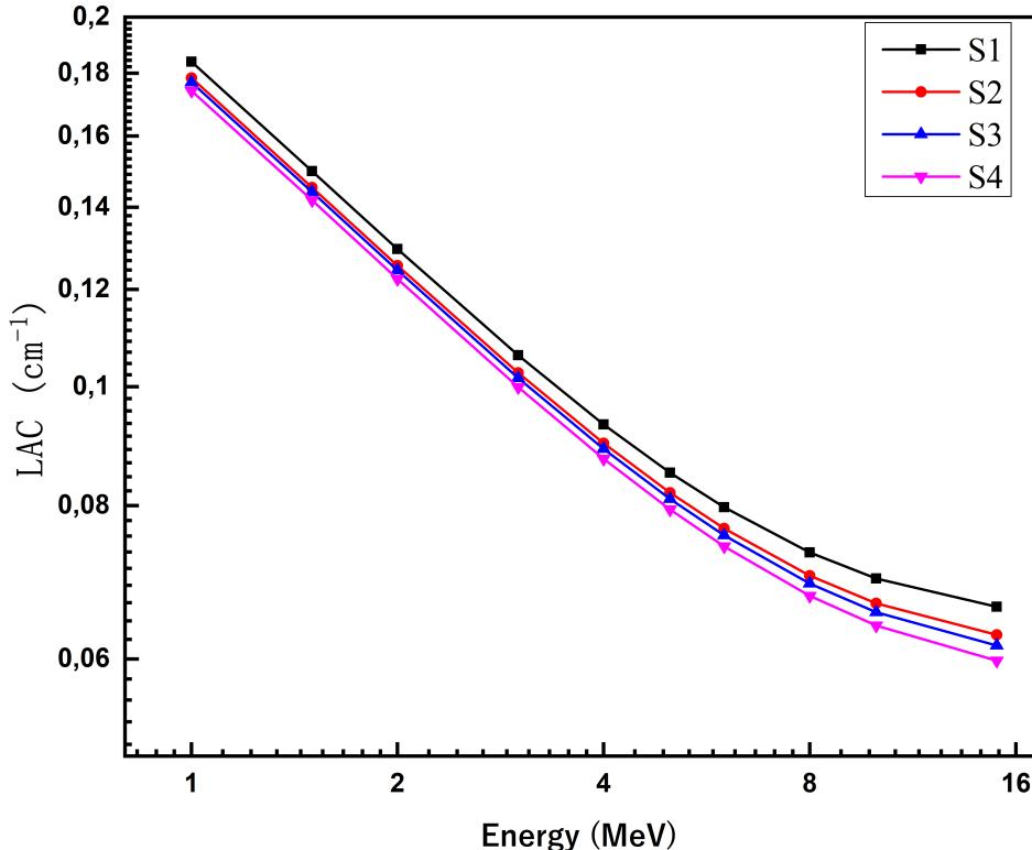
**Figure 1.** Variation of the linear attenuation coefficient (LAC) with photon energy (1–15 MeV) for calcium aluminosilicate glass samples S1–S4, simulated using Phys-X/PSD.
