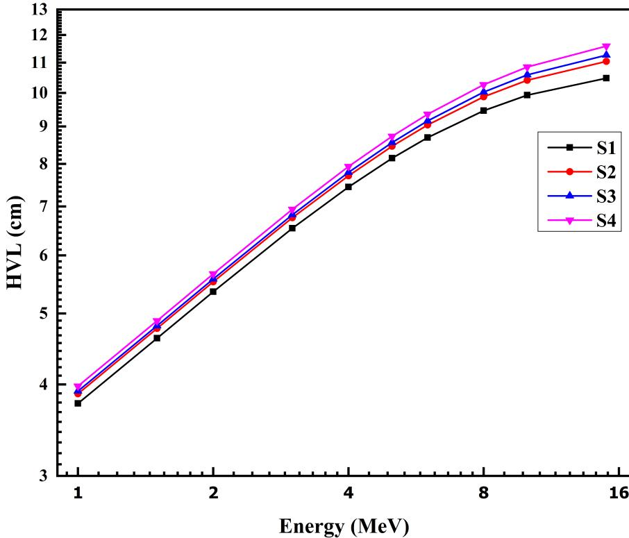
**Figure 2.** Variation of the half-value layer (HVL) of the calcium aluminosilicate glass system across photon energies ranging from 1 to 15 MeV.
