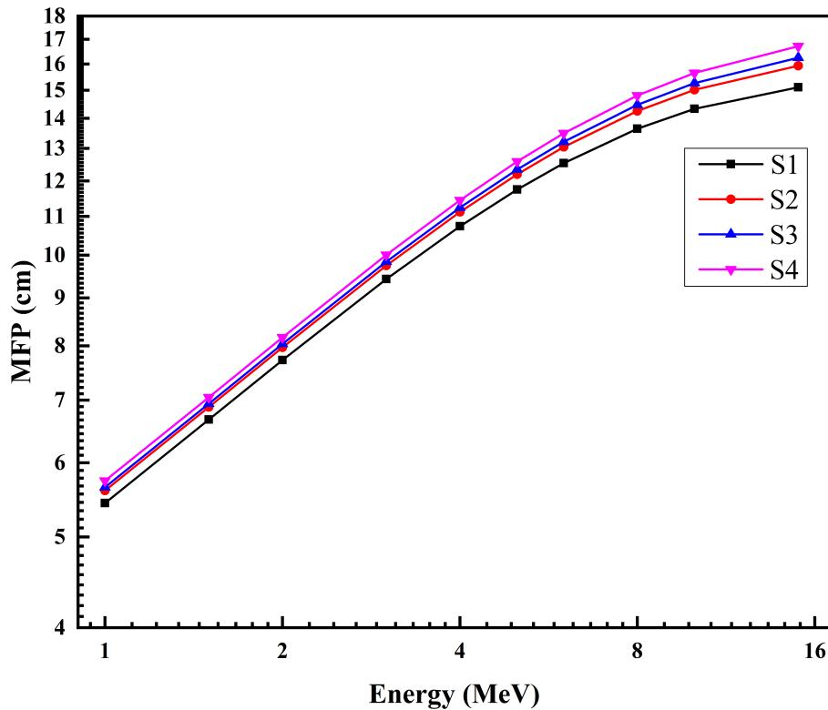
**Figure 3.** Mean free path (MFP) of the calcium aluminosilicate glass systems as a function of photon energy in the 1–15 MeV range.
