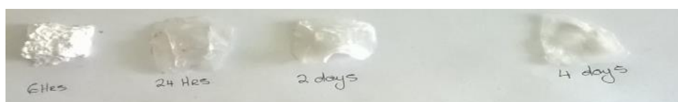
Figure 5: TONC paper at 6, 24, 48 and 96 hours of oxidation time
