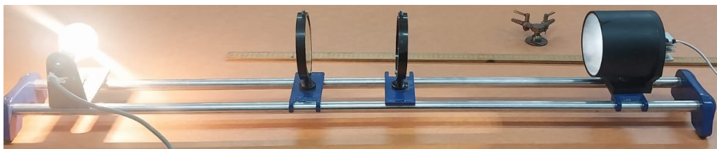
Figure 2: Visual comparison between older incandescent light technology and the new LED based light source as implemented on the optical bench experiment.
